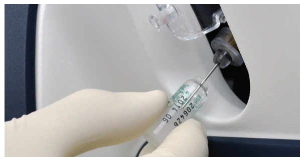
QC proficiency ampoules can be sampled without adapters.
